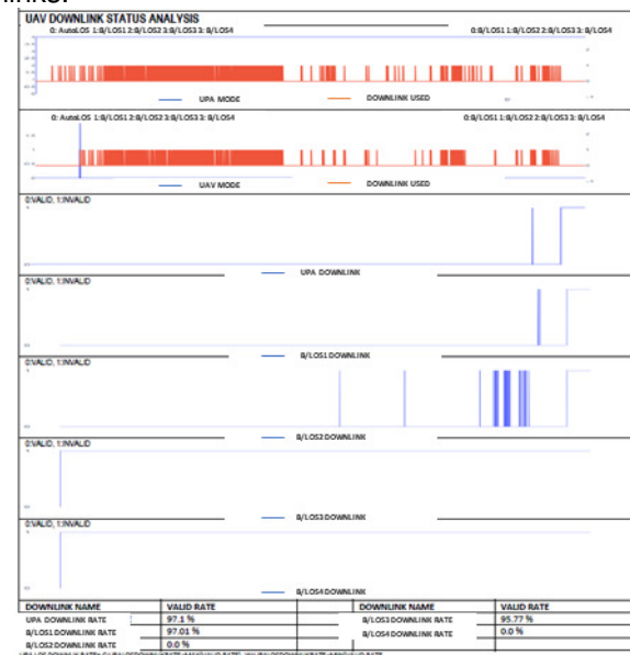
Fig. 28. UAV downlink status analysis
