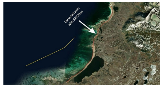
Fig. 1. Graph of spoofed trajectory in the water (yellow) and true trajectory (orange) along a coastal road. Source SBG Newsletter May 2026
