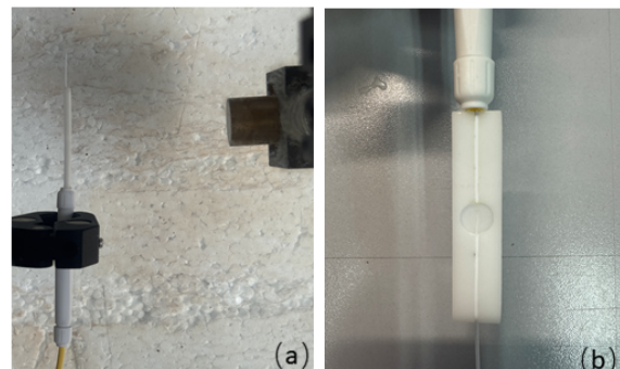
Fig. 5: (a) Experimental diagram of a sound wave incident vertically on PS-FBG and (b) Physical diagram of the sensitized structure package.
