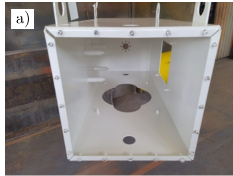
Fig. 1: Illustration of the fabricated sea chest used in the experimental field tests.
