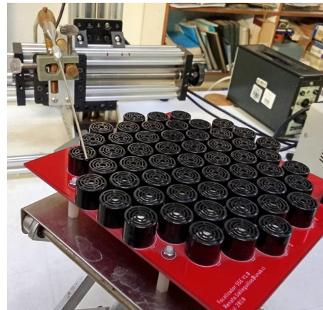
Fig. 2: Acoustic field characterization setup, showing an array of ultrasonic transducers. On the left edge of the array, the tip of the microphone waveguide can be distinguished, which is arranged horizontally and attached to the two-dimensional scanning system.
