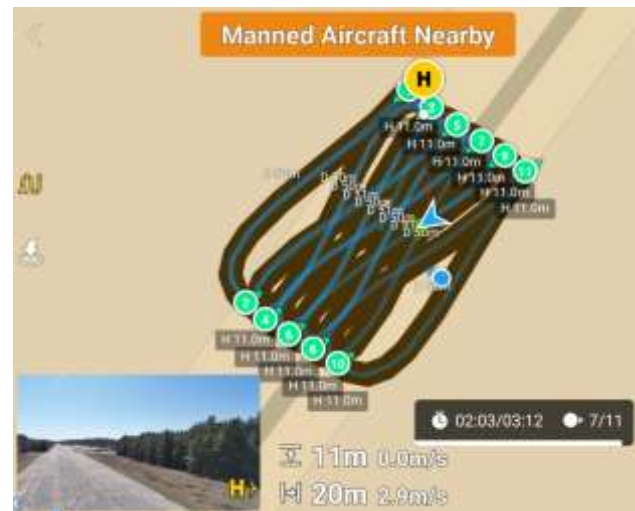
Figure 2 Preprogrammed automatic UAV flight mission path with a constant speed and altitude.
