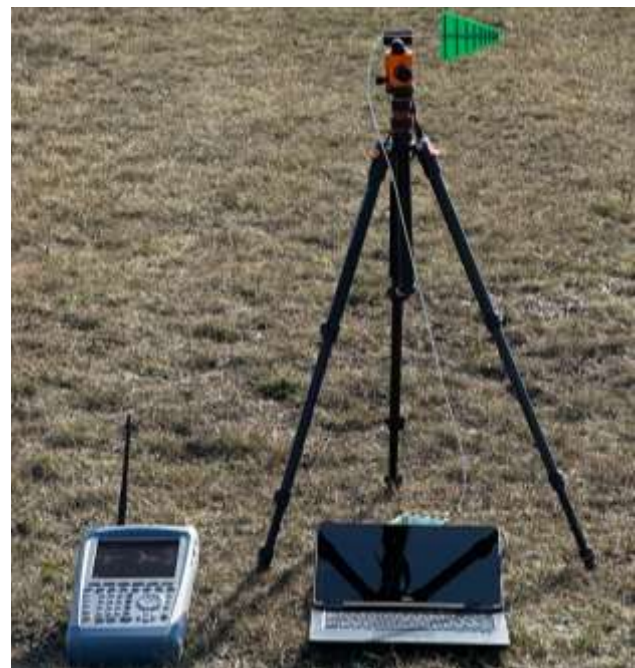
Figure 3 SDR-based jamming hardware with a high-gain directional antenna and Rohde&Schwarz FSH8 spectrum analyzer.
