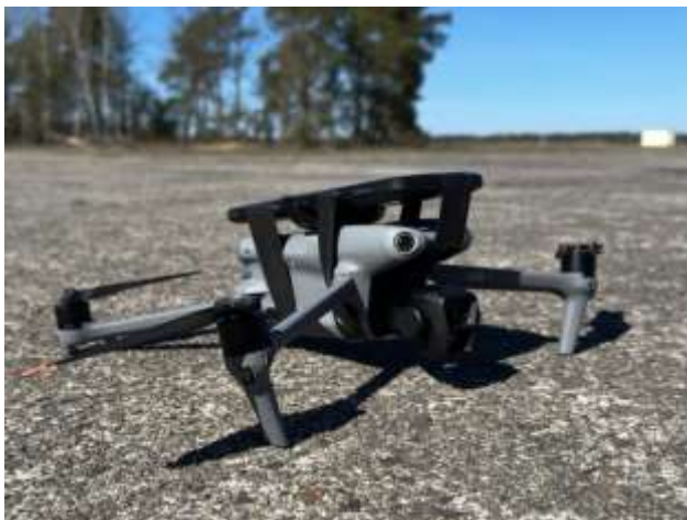
Figure 1 Quadcopter UAV fitted with a Rohde&Schwarz QualiPoc Android network quality testing device.
