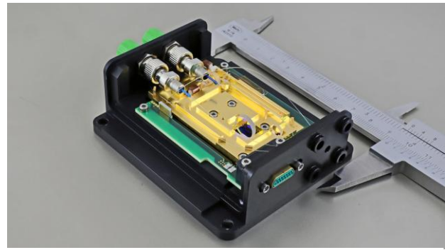
Figure 2 Inside view of an SPDC module with integrated fiber connectors and internal fiber coupling of the signal radiation.
