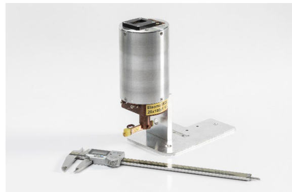
Fig. 2. ELSOPULS IIM2k impulse-magnetization head (Source: ELSOMA GmbH)
