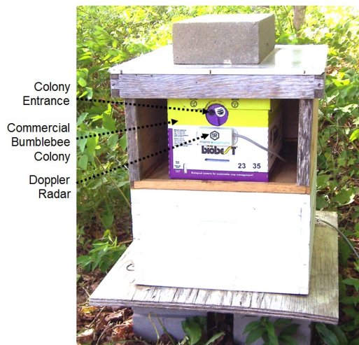
Fig. 1. Bumblebee colony with radar sensor
