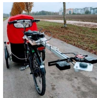
Fig. 1. Multi-sensor pothole detection system mounted on a bicycle at a height of 0.8 m
