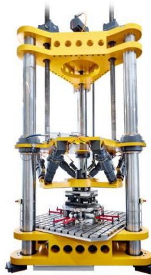
Fig. 1. Multi-component standard machine for uniaxial loading and mixed loading, performing forces moment-free and moments force-free
