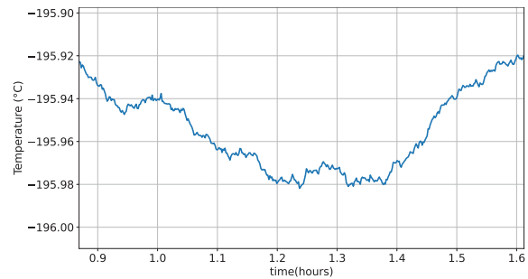
Fig. 2: The time dependence of the measured temperature of liquid nitrogen shows a stable minimum temperature of -195.98^{\circ}\text{C} .
