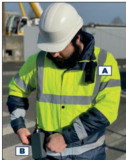
Fig. 3. Sensor used by worker consist A – sensor head, B – electronic board with battery.
