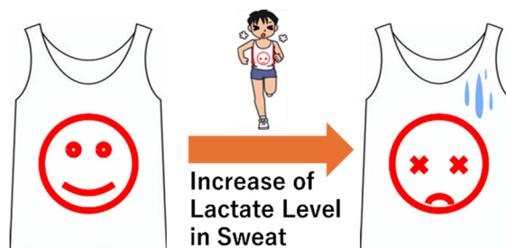
Fig. 1 Concept of our wearable lactate sensor with dynamic visual pattern responses
