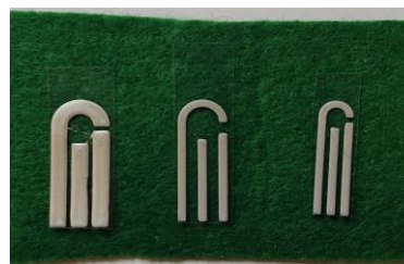
Fig 1. Printed electrochemical sensor with 3 electrodes. From left to right the parameters for the electrodes changed are: 2mm of thickness and 1 mm distance ( d1t2 ), 1mm thickness and 2mm distance ( d2t1 ) and 1mm thickness distance ( d1t1 )
