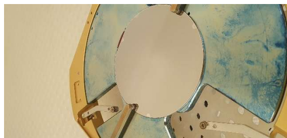
Fig. 5: 100mm SiC-Insulator-Silicon carrier after bonding.
