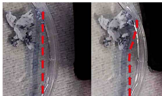
Fig. 4. The effect of the magnetic field on the flow channel with the blue coloured water line, without the presence of the magnet (left) and with the magnet in its proximity (right).
