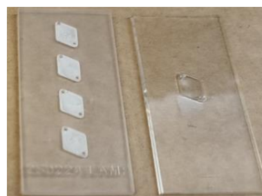
Fig. 2. Ready-to-use chips for RT-LAMP: 3D printed (on the left) and all-glass (on the right)
