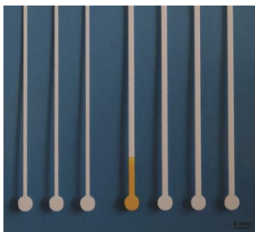
Fig. 2. Photograph of printed straight capillary microfluidic channels. 2 seconds after a diluted inkjet ink was dropped onto the inlet of the central channel, and a colored paper was placed underneath for photo taking.
