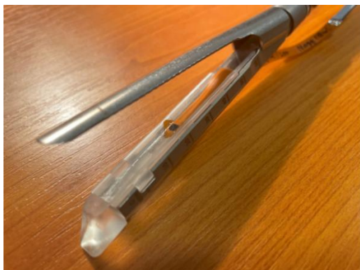
Figure 1. 3D printed stapler cartridge with the integrated MEMS force sensor
