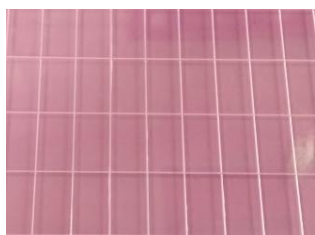
Fig. 1. The uniform thin film-based LSPR sensor on a glass wafer
