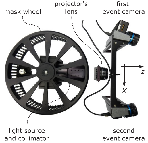
Fig. 3: Measurement part of our experimental setup. Two event cameras observe a scene beyond the right edge. The mask wheel is illuminated from the light source within. Rotation causes the projected images of the mask to form moving contrast edges in the measurement volume. These sample the scene and trigger event measurements in the event cameras.
