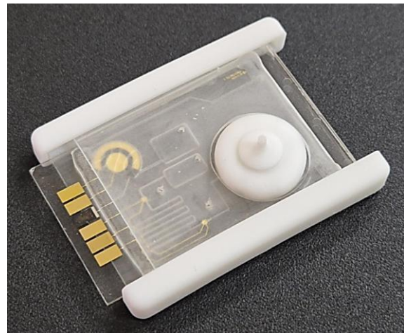
Fig. 2. Photograph of the assembled bimodal sensor cartridge.
