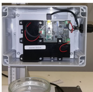
Fig. 1. A) Optical pathway of the confocal fluorescence detector. B) View of the assembled Detector.
