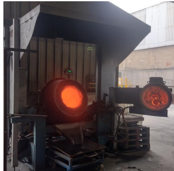
Figure 1: Application scenario showing the rotary furnace with 10 kg capacity for scrap characterization.
