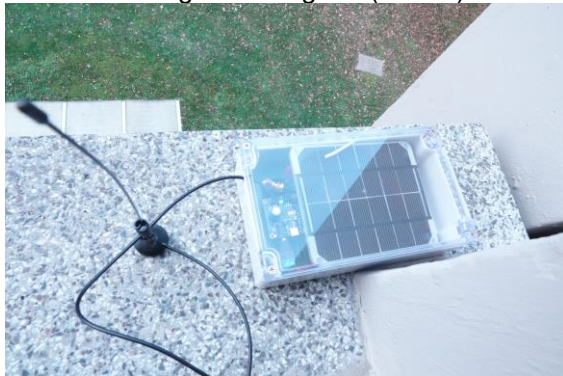
Abb. 5: Autarkes mobiles Multisensorbox
