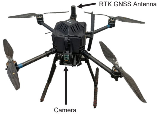
Fig. 1: UAV equipped with camera, RTK GNSS antenna, and Nvidia Jetson, to estimate the distance.
