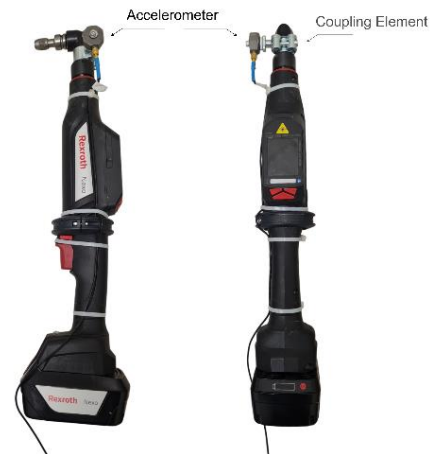
Fig. 2: Handheld electric screwdriver with a piezoelectric accelerometer non-destructively mounted near the bit holder to capture process-related vibrations.
