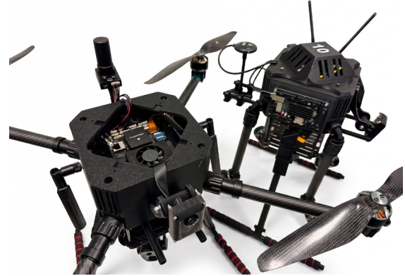
Fig. 1 UAV experimental setup showing Nvidia Jetson, Pixhawk 6X, and Quectel RMU500EK 5G modem mounted on a Holybro X650 Frame.
