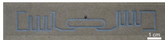
Fig. 4. Optical image of the zinc antenna printed on PHX and assembled to an UHF RFID chip.
