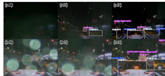
Fig. 3. Sequential snapshots of the electrokinetic removal of contaminants on an optical sensor and the restoration of object recognition: (a) Solid particles; (b) Droplets.
