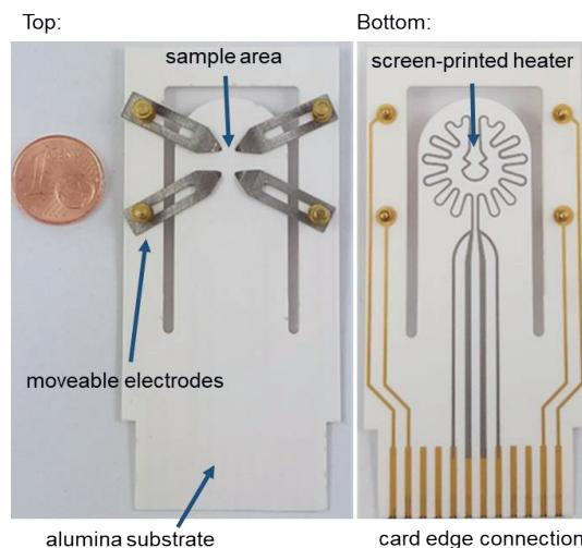
Fig. 1. Sample holder for Hall and conductivity measurements with a screen-printed heater
