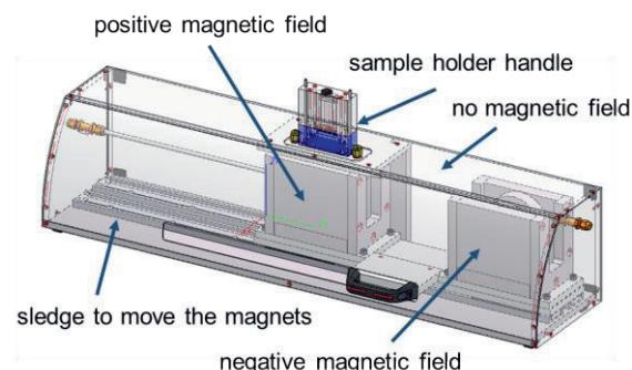
Fig. 2. Measurement setup with two moveable permanent magnetic yoke systems with  $\pm 760$  mT
