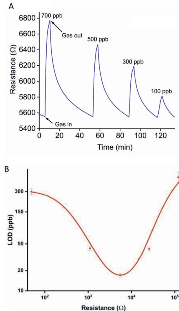
Fig. 1. A) Resistance change as a function of time upon exposing a sensor based on a percolation network of PPy to 700, 500, 300, and 100 ppb of ammonia. The sensor response is instantaneous and reversible. B) The limit of detection (LOD) for sensors with different starting resistances, corresponding to different points along the percolation curve. A LOD of  $18 \pm 2$  ppb was achieved at the optimum, which is found at a resistance value corresponding to the steep part of the percolation curve.
