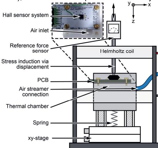
Figure 3: Schematic and photograph of automated measurement setup for calibrating Hall-stress-temperature sensor systems. Induction  $B$ , temperature  $T$ , and stress  $\sigma$  are applied via Helmholtz coil, air stream into thermal chamber, and mechanical loading mechanism, respectively.
