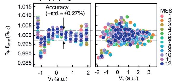
Figure 6: Hall sensitivities of 12 MSS compensated with the best 4<sup>th</sup>-order polynomial  $f_{\text{comp}}$  with only 6 parameters.
