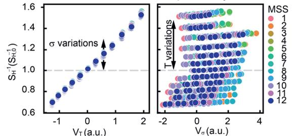
Figure 4: Measured calibration data:  $T$  and  $\sigma$  dependent, uncompensated inverse Hall sensitivity of 12 MSS vs. respective output signals  $V_T$  (left) and  $V_\sigma$  (right) of  $T$  and  $\sigma$  sensors.
