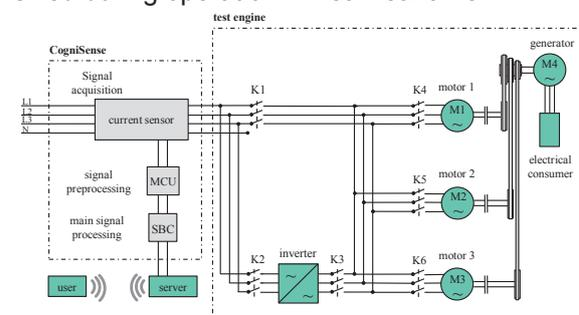
Fig. 1. Schematic of test engine and "CogniSense"
