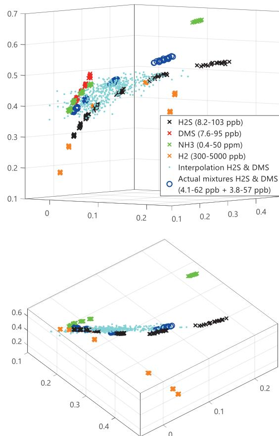
*Fig. 2.* 3-dimensional representation of the (6-dimensional) interpolation (cyan) between two classes ( $H_2S$  and DMS) from two perspectives. Individual gases and their interpolation form one plane, on which the actual mixtures of both gases (blue) lie also. Only a mixture with higher concentrations (highest blue data points) lies outside the interpolated class.
