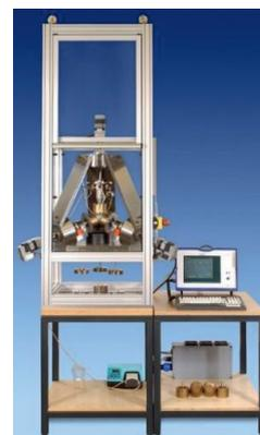
*Figure 1 Polishing machine to manufacture high-precision spheres*
