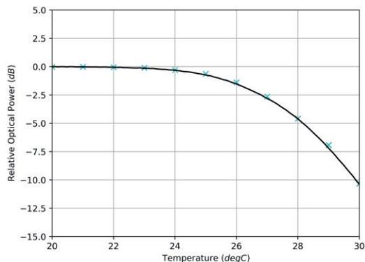
Fig. 4. Relative optical power at different temperatures vs. reference derived from 22 °C curve (black).
