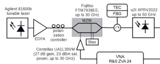
Fig. 1. Block diagram of the experimental setup.
