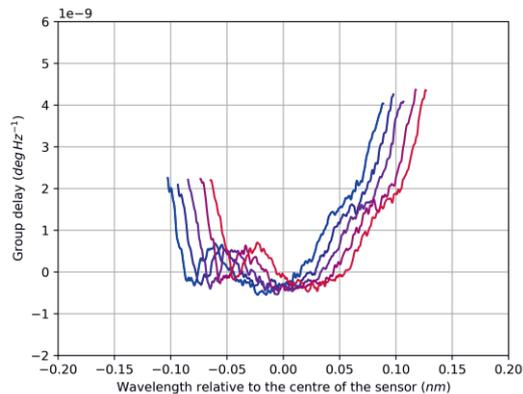
Fig. 3. Group delay characteristic of FBG derived from el. phase from 21 °C (blue) to 25 °C (red).
