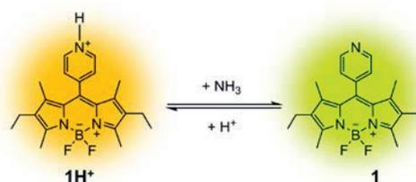
Fig. 1. Scheme of sensor dye **1** and the fluorescence change ( $\lambda_{ex}$  365 nm) in presence of ammonia.
