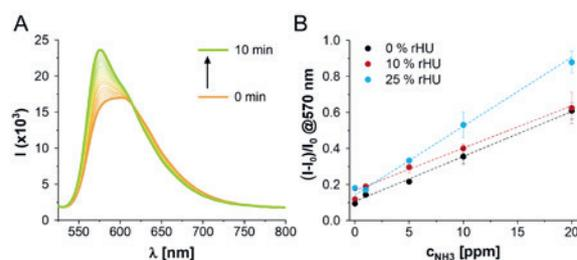
Fig. 3. Time dependent response in presence of 20  $\mu\text{mol mol}^{-1}$  ammonia (A) and fluorescence change at 570 nm at different ammonia concentrations and relative humidity after 10 min (B) measured with the developed FS-GIMMD ( $\lambda_{ex} = 500 \text{ nm}$ ).
