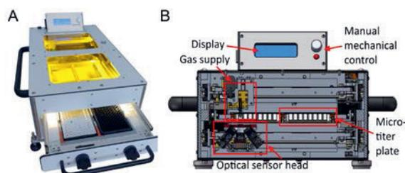
Fig. 2. Picture (A) and a scheme of the main mechanical parts (B) of the FS-GIMMD prototype.
